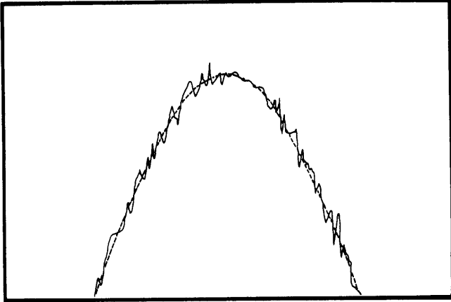
Figure 2-6. SIGNAL VOLTAGE WITH CONVERTER NOISE
